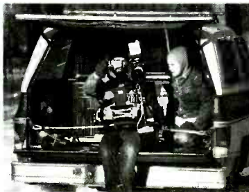
Cameraman Steve Dubin with CP-16R and STEADICAM. STEADICAM converts virtually any vehicle into an "instant" camera platform.
